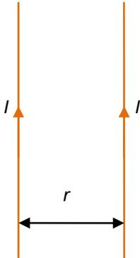
The force per unit length on each wire is  $f$ . The separation and the current in each wire are all doubled. What is the new force per unit length on each wire?
