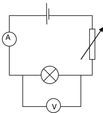
By measuring the resistance of the light bulb and knowing the temperature coefficient of resistance of the filament the temperature of the filament was established. The power of the light bulb was found by multiplying the voltage by the current.
